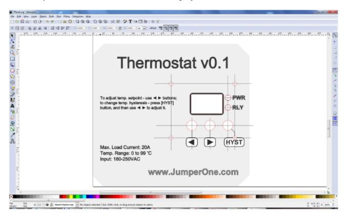
And this is how front panel label looks like when it's done. Btw, I've messed it up a bit - I should've made display and LED centers white, instead of gray.
