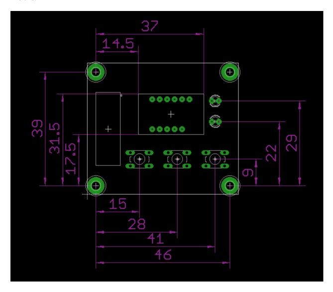
This kind of information about board dimensions and components placement would be essential for designing front panel labels, where you need to know where all the switches, buttons, displays and other components are.
